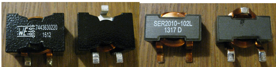
Figure 19: Würth Elektronik HCF2013 with PQ core (39) and Coilcraft SER201X with a hybrid PQ/EE core
