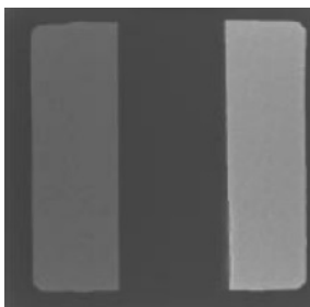
Figure 2.2: Dark current effect on an image sensor [H + 00]
