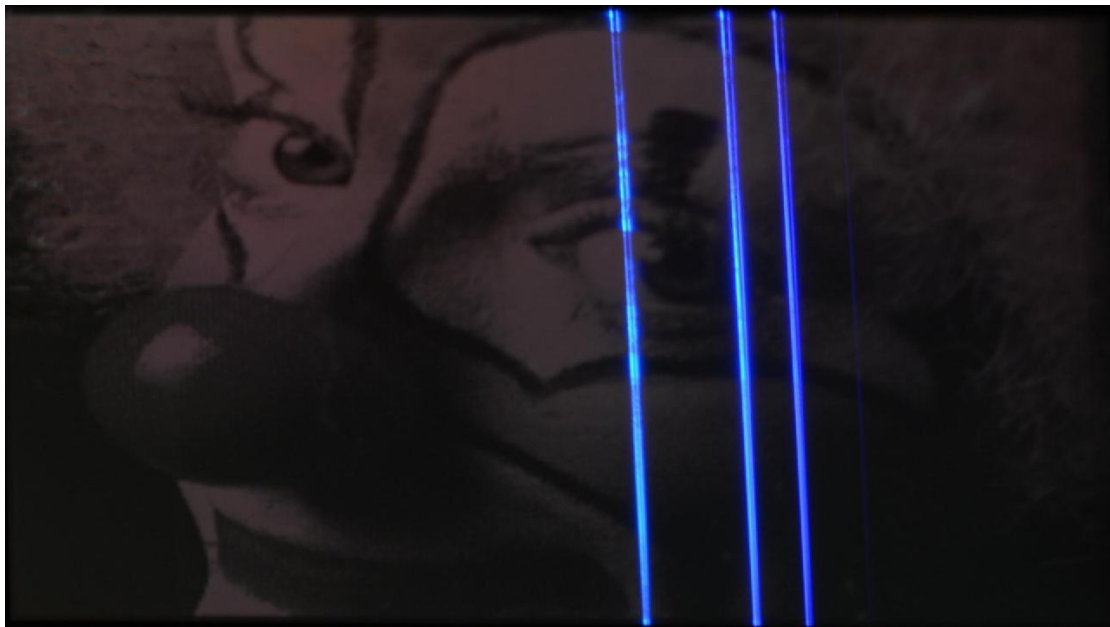
Figure 19: The DMD chip surface uploaded with a gray scale picture of a clown reflects a lower percentage of the lines from whiter portion and vice-versa.
