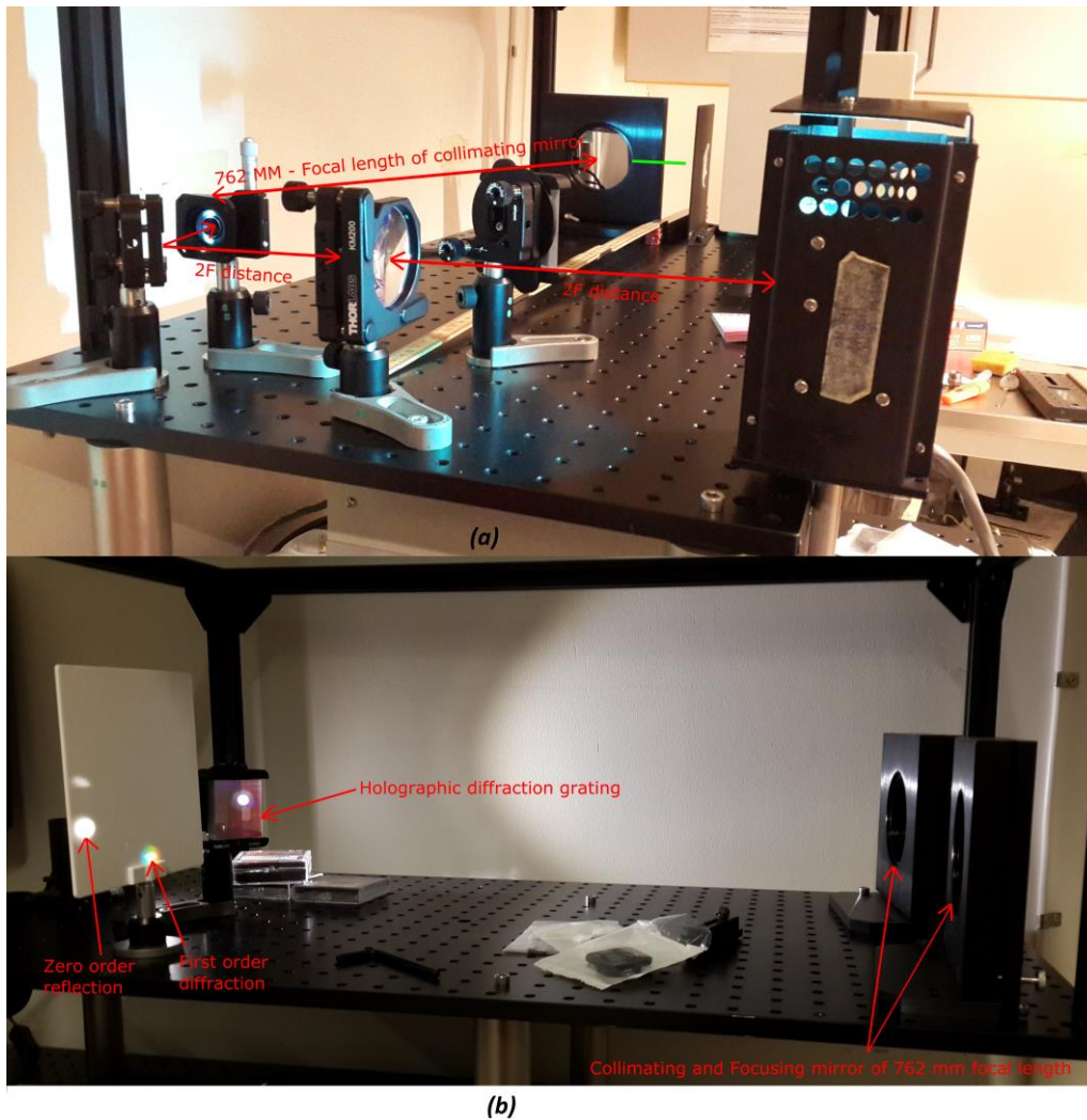
Figure 8: (a) Image formation of spectral lamp at the entrance slit. The collimating mirror was placed at a focal length distance from the slit. The Green horizontal line representing the height of the focal plane defined inside the spectrometer. (b) Side view to show the diffraction grating, collimating and focusing mirror, focusing the 0 th order and first order diffraction.
