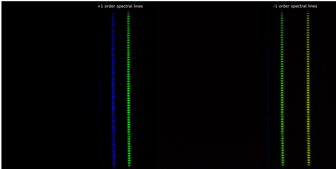
Figure 13: Two captured pictures put together showing the spectral lines of +1 and -1 diffraction order with superimposed periodic shadows.
