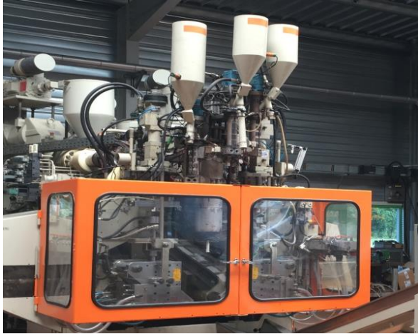
Extrusion blow-molding machine for plastic bottles
