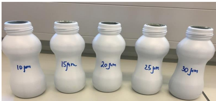
Nutricia bottles measured by supplier and at Nutricia laboratory. 5 different thicknesses of EVOH – 10, 15, 20, 25 and 30 micron
