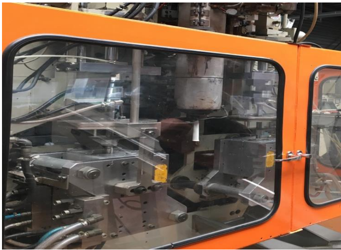
Plastic is melted and extruded into a hollow tub
