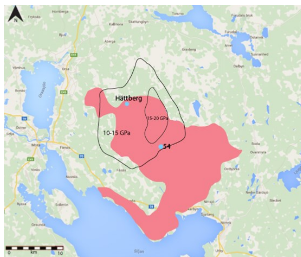
Figure 16 Map over the Siljan crater area. Pink area indicates bedrock of Järna-granite type, blue dots show locations for sample 54 and the Hättberg-samples. Black lines show the different estimated pressure-ranges (Modified and based on Holm et al 2011)
