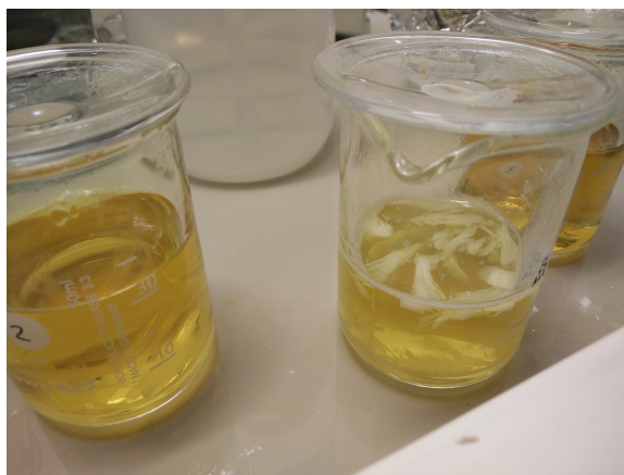
Figure 11: Qualitative representation of the degree to which the cellulose was extracted (white strands are the cellulose)
