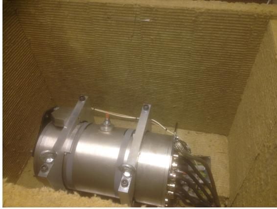
Figure 5.15: The PMSM placed inside an isolated cage for the purpose of investigating thermal dependency.
