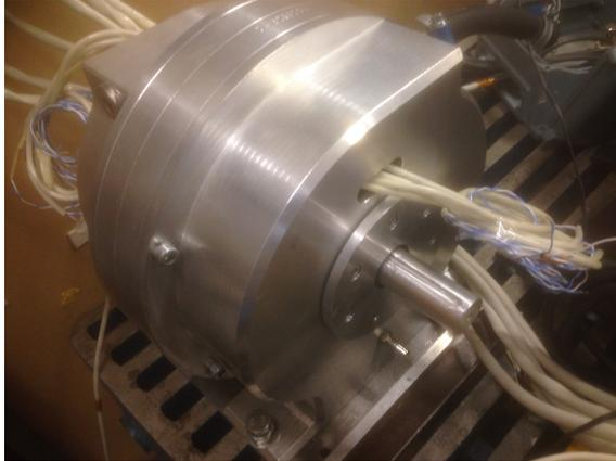
Figure 4.2: Picture of the PMSM under test.
