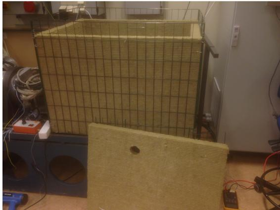
Figure 5.16: The isolated cage containing the PMSM.
