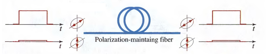
(b) When single polarized radiation instead is transmitted into polarization-maintaining fiber the power remains in the same polarization.
