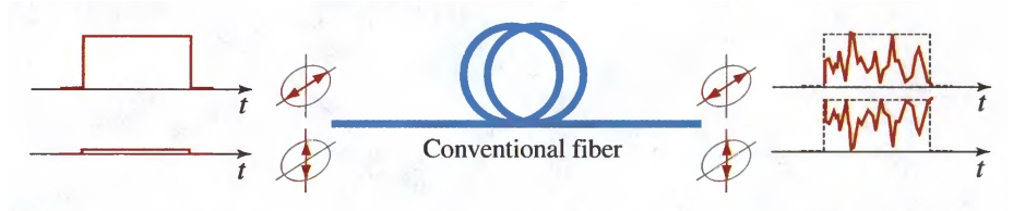
(a) A signal passes through a non-polarization-maintaining fiber. At the end the total optical power remains the same but it is randomly distributed over the two different polarizations.
