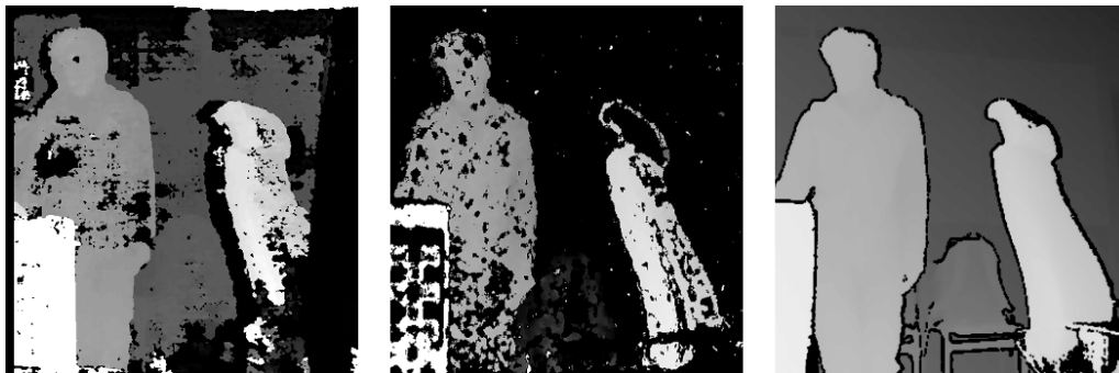
Figure 2.7: Depth image comparison. Left: Passive stereo with color cameras, Center: RealSense (Hybrid stereo with infrared cameras), Right: Kinect One (time-of-flight, phase-shifting)
