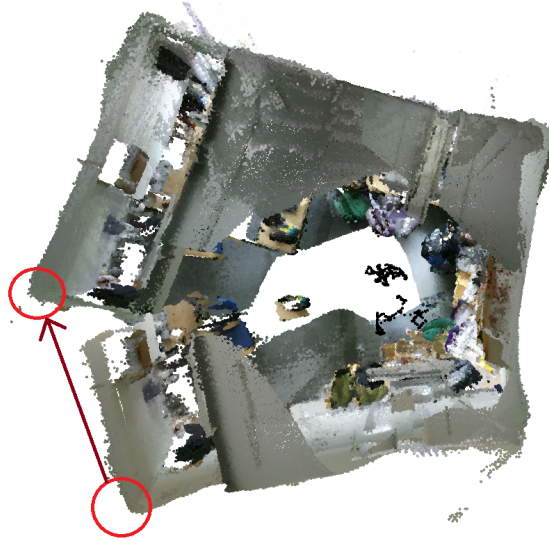
Figure 3.5: Accumulated error from around fifty registrations resulting in heavy drift from a 360° scan of a rectangular room, with drifted corners marked with circles.
