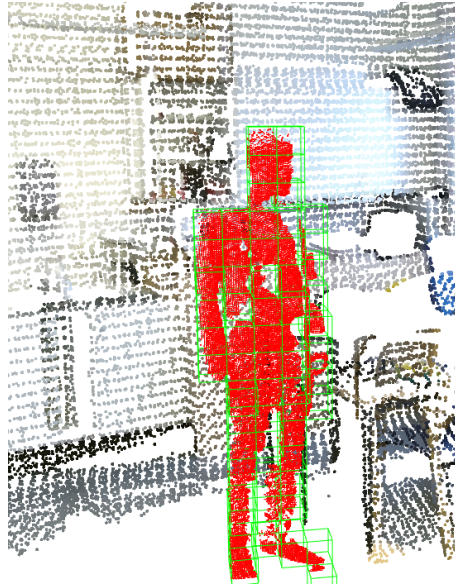
Figure 5.3: A high density region of interest detected from data captured by a Microsoft Kinect One.
