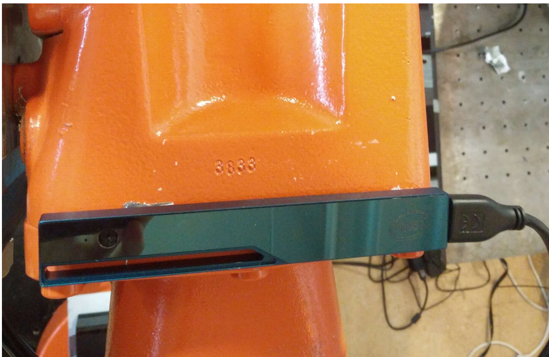
Figure B.3: The mounted Intel RealSense on robot link 4.
