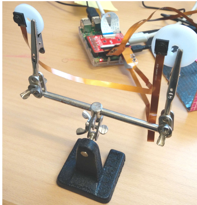
Figure 2.2: A setup of a stereo vision system using regular color cameras and a Raspberry Pi as computational unit
