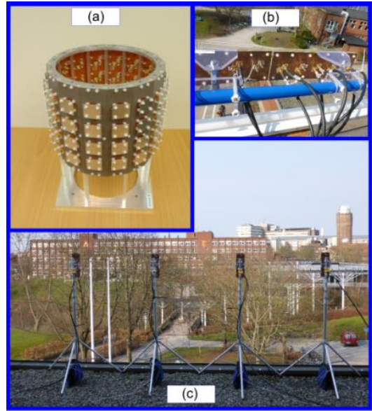
Fig. 1. Antennas at the MS and at the BS. (a) MS antenna: stacked uniform cylindrical array with 64 dual-polarized antenna elements arranged in four rings. (b) BS antennas: co-located arrangement used in setup-II with inter-patch spacing of \lambda/2 (back view). (c) BS antennas: mounted on a tripod to facilitate adjusting the inter-element spacing for setup-I, the photo is with inter-element spacing of 1 m (back view).
