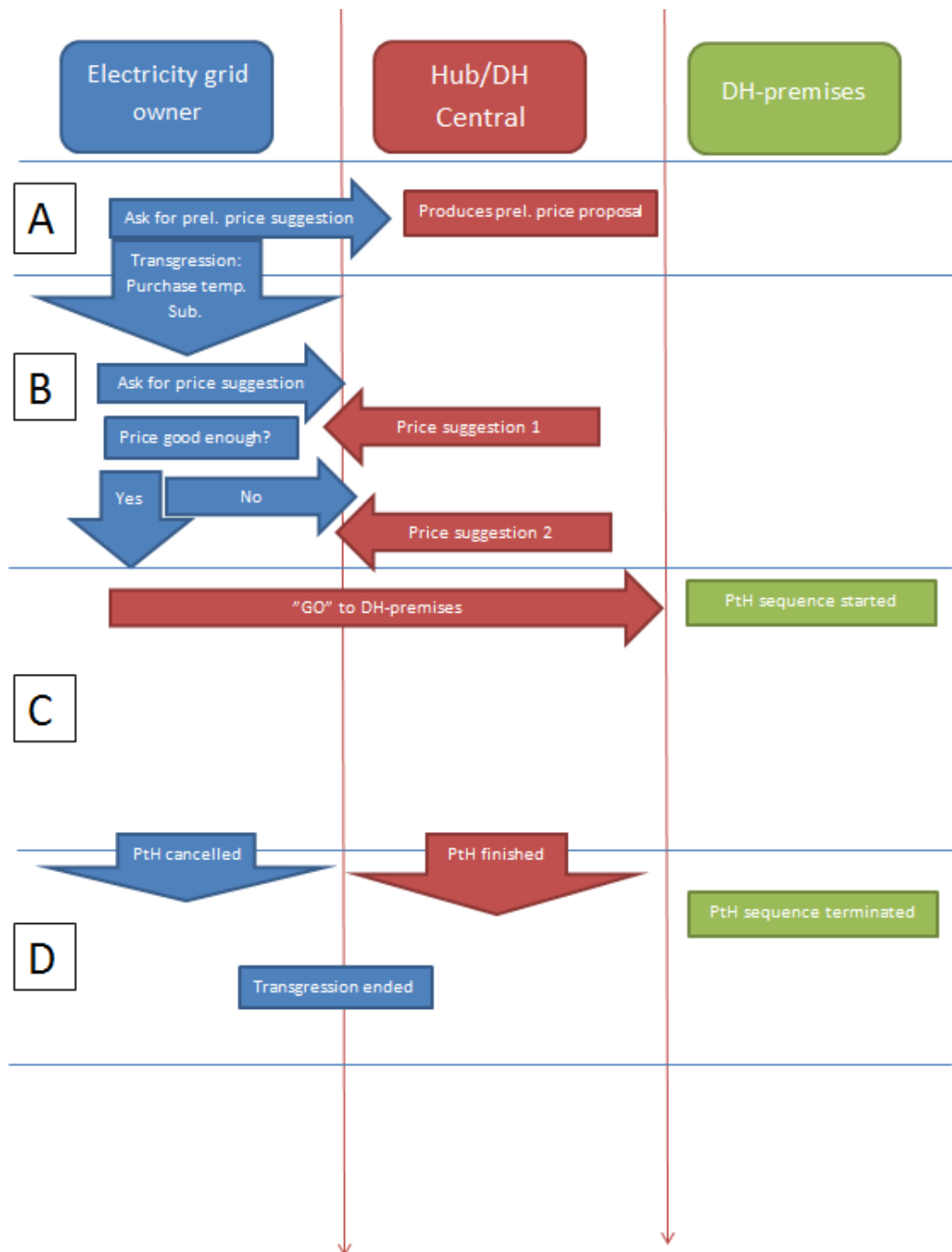
Figure 8.3: In this figure the process flow of the agreement framework is presented. Starting with alerting the parties in section A, making price and volume suggestions in B, considering the opt-out in C, and then terminating or finishing in D.
