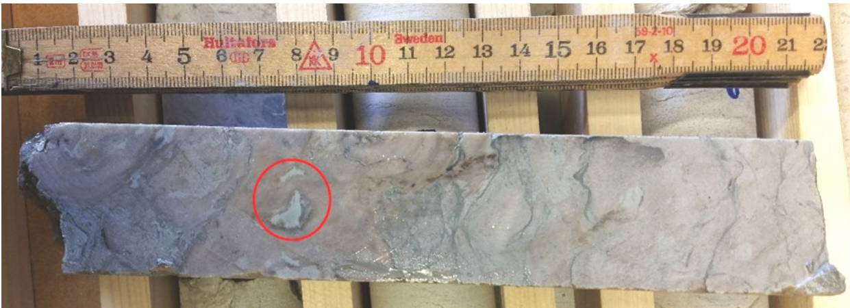
Fig 19. A sample of reef limestone from the drill core (about 24 m down). A typical marl-pocket is marked with red.
