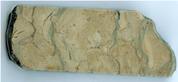
Fig 18. A sample of reef limestone from the core (about 24 m down).
