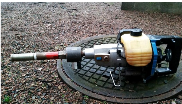
Fig 1. A picture of the handheld drill used to collect the Samples. Photo: Jessica Jennerheim
