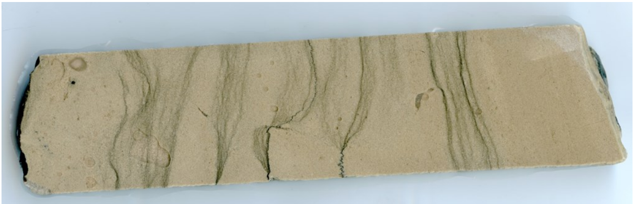
Fig 12. A sample of calcarenite from the Core (about 19 m down). Note the clear lamination and stylolites.
