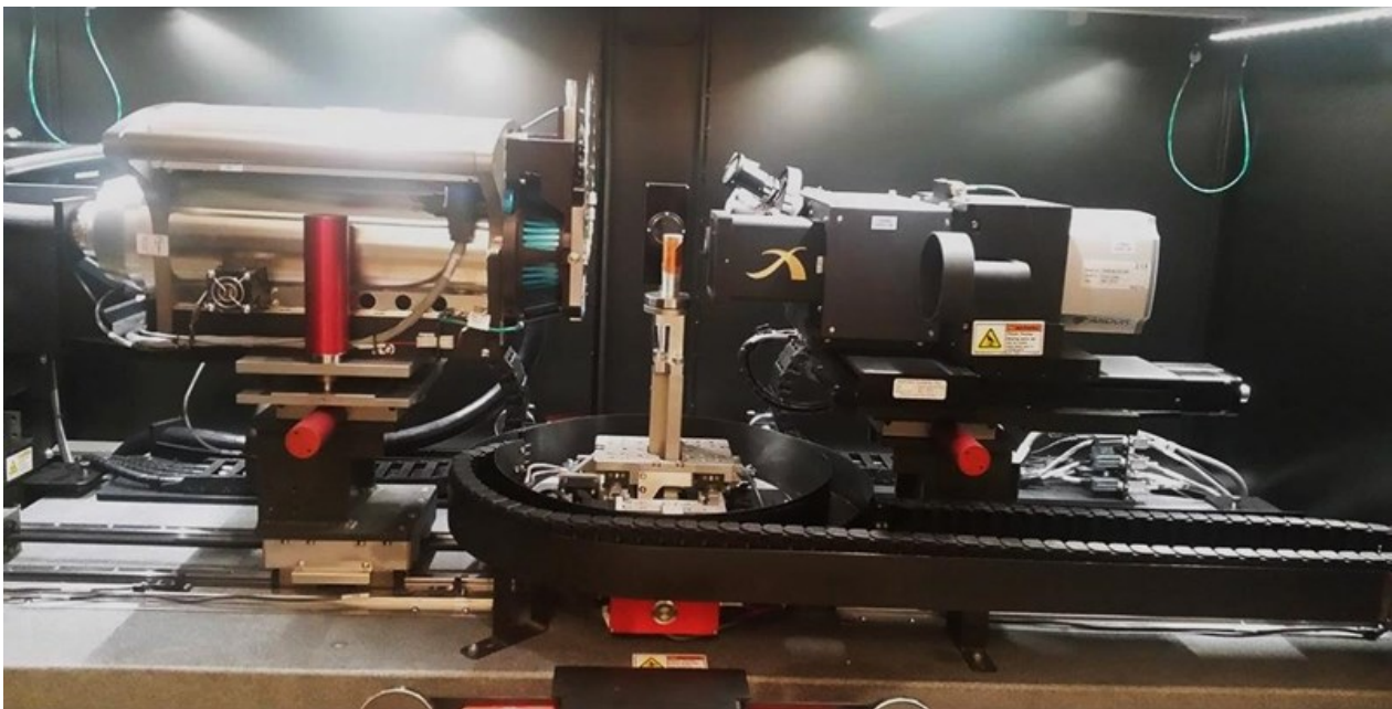
Fig 2. The CT scanner used in this study. Photo: Jessica Jennerheim
