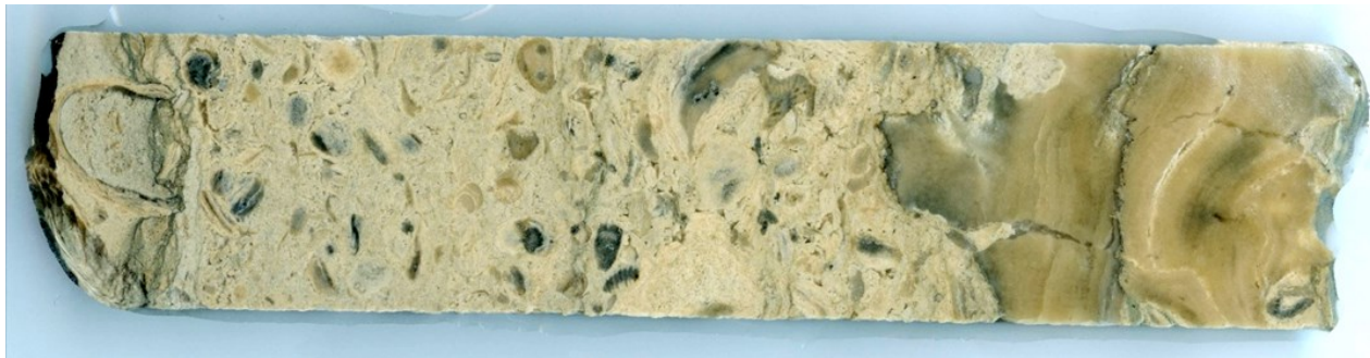
Fig 10. A sample of calcilutite from the core (about 28 m down).
