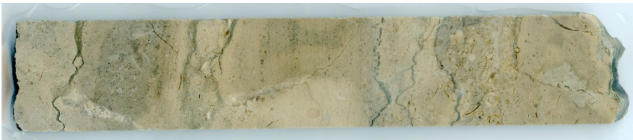
Fig 14. A sample of stromatoporoid limestone from the core (about ten meters down). The stromatoporoids are light beige in the picture.
