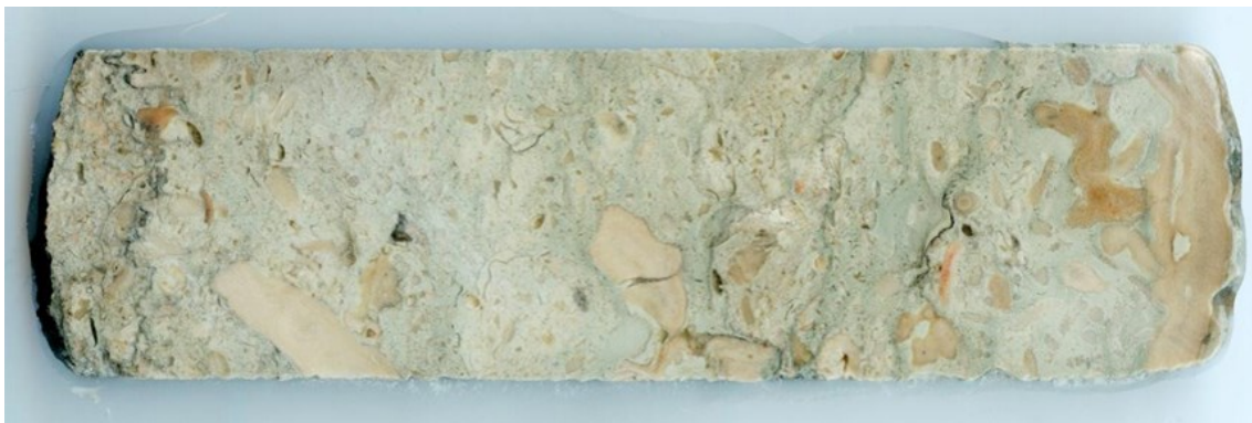
Fig 16. A sample of fragment limestone from the core (about 6 m down).
