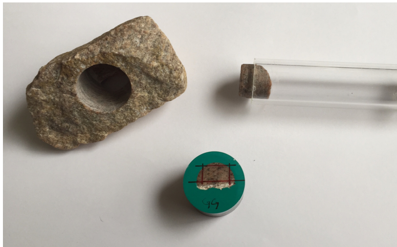
Figure 3.9 - Red gneiss rock, plastic tube and a pellet
