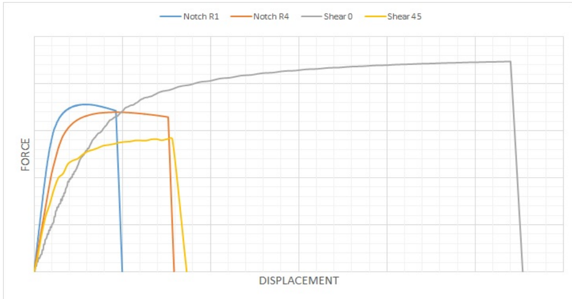
Figure 13: Force-displacement curves for Notch R1, Notch R4, Shear 0^\circ and Shear 45^\circ .
