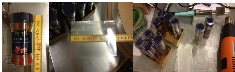
Figure 12: Process of placing the plastic sleeve manually.
