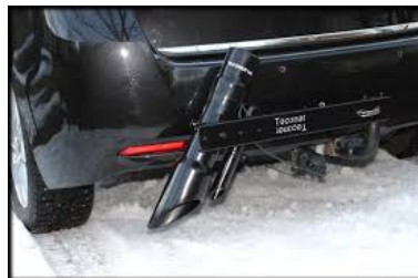
Figure 8: Attachment of the RCM411 sensor to a car.
