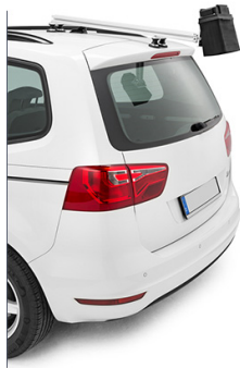
Figure 6: Attachment of the MARWIS sensor to a car.
