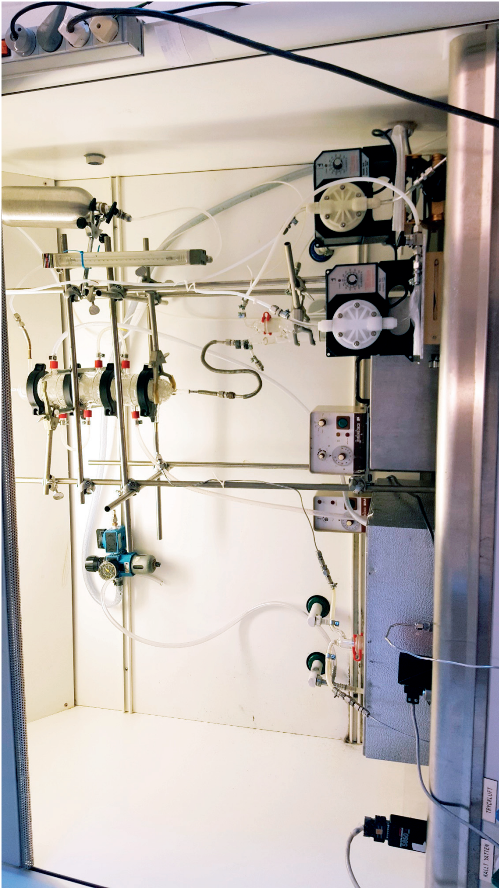
Figure 38. Absorption setup installed within the fume hood. The laboratory work has been divided into the following operations:
