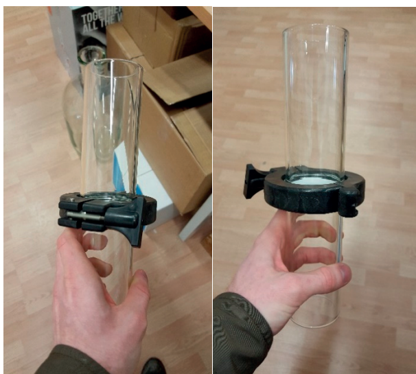
Figure 19. Plastic clamp for connecting the column segments.
