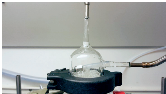
Figure 31. Rubber tube with stop to introduce the liquid at the center of the column.
