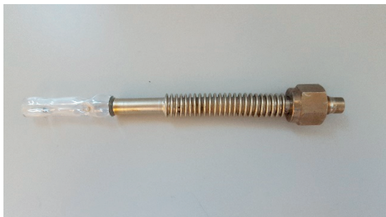
Figure 20. Glass-metal connector for gas and liquid inlets and outlets.
