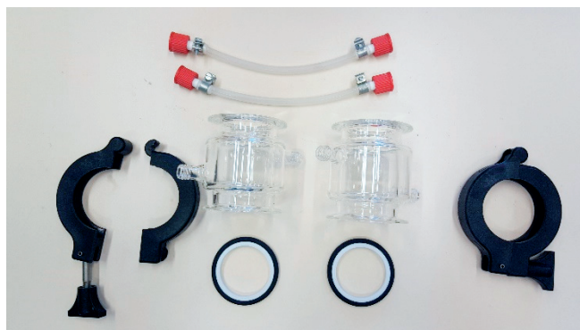
Figure 22. Parts for the absorption column, including jacketed glass segments, Teflon gaskets, plastic clamps and GL14 plastic connectors.
