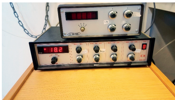
Figure 33. Instrument to control the mass flowrate of the two gases.
