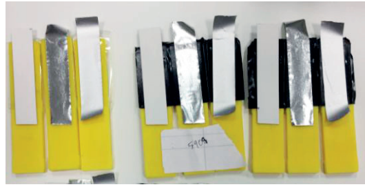
Figure 5.9 Samples with reinforced aluminium as peel arm
