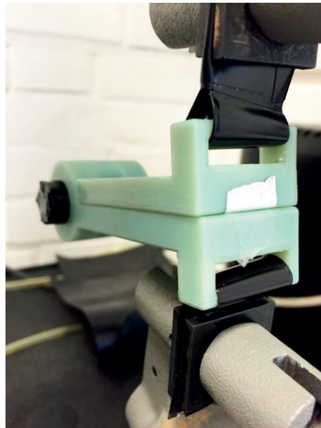
Figure 5.10 The DuckFace with taped sample mounted in the tensile tester
