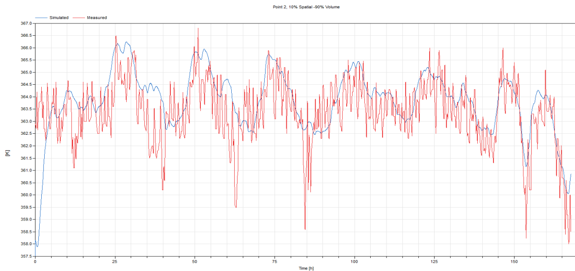
Figure 4.12. A graph of the temperature from the simulation and the measured results. The red line show the measured temperature and the blue show the simulated temperature using a spatial operator pipe with split-ratio of 0.1 .
