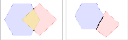
Figure 4.6. The intersection of two polygons boundaries can consist of both 0-dimension geometries (points) (left figure) and 1-dimension geometries (lines) (right figure) (Partly based on GeoTools 2016).
