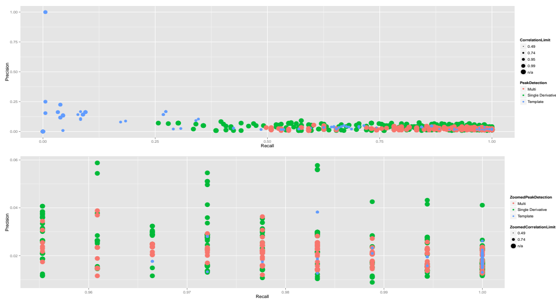
Figure 3.8: Performance of the different peak detection methods along with the threshold value of the template method on the medium noise file. The first graph is a overview and the second is zoomed in on high recall. Each dot represents a parameter combination and show the performance in recall and precision.
