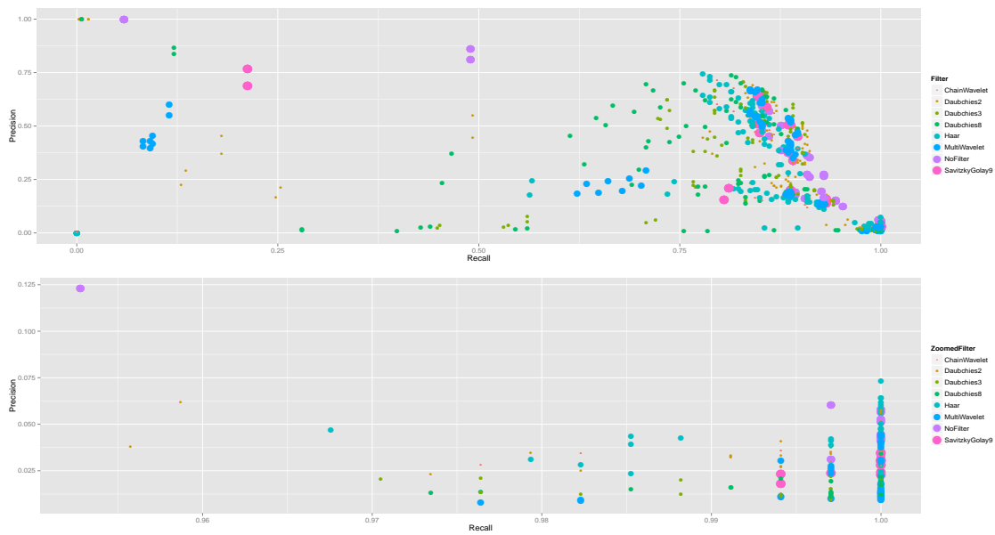
Figure 3.4: Performance of the different filters on the low noise file. The first graph is a overview and the second is zoomed in on high recall. Each dot represents a parameter combination and show the performance in recall and precision.
