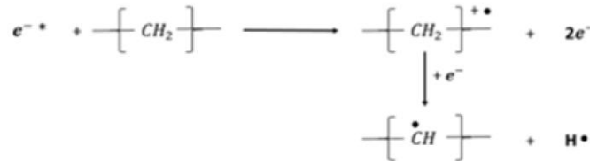
Figure 9 The electric breakdown mechanism of polyethylene
