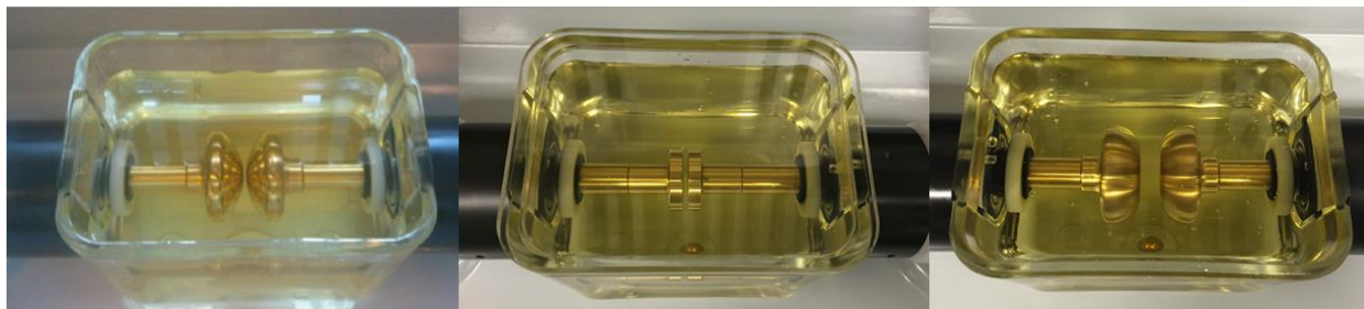
Figure 19 The oil bath in the BA 100 breakdown analyzer with different electrodes that could be used to test different materials DBS with AC breakdown; Mushroom shaped electrode (left), Flat shaped electrode (middle) and Rogowski shaped electrode (right). The Rogowski shaped electrode geometry was used for AC breakdown tests and the Mushroom shaped geometry was used for Lightning impulse tests
