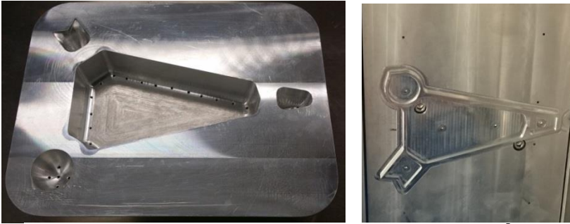
Figure 18. Mould for forming (left) and sealing (right) on Multivac ® machine
