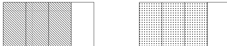
Figure 3.5: Worst-case register allocation of B and C , where B is allocated to the left register and C to the right register.
