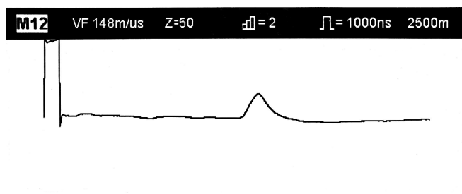
Figure 77: TDR-Result, K70 signal.
