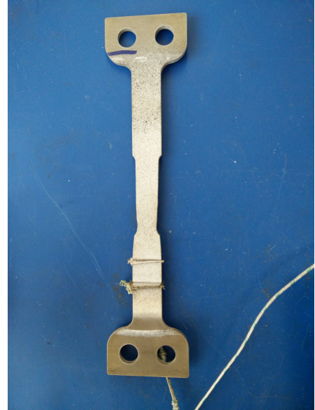
Figure 8: The figure shows the painted white background and the stochastic black pattern on the specimen. One can also see the thermo-couple that is welded on the back.
