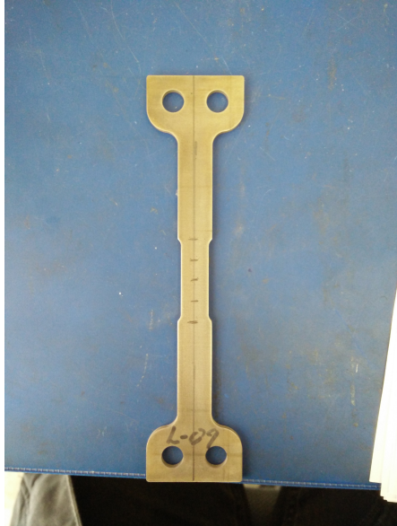
Figure 7: Figure shows the sandblasted but not yet painted specimen where measurements of thickness and width has been done.
