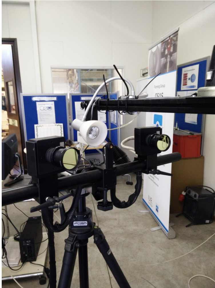
Figure 11: Figure shows the cameras and lights that take the images for the ARAMIS camera and strain measurement system.
