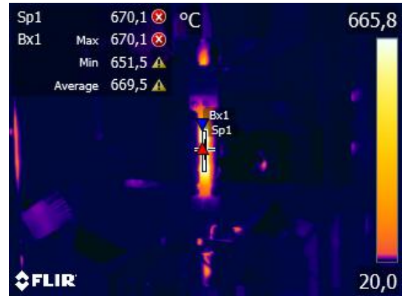
Figure 15: Figure shows specimen L06 which were heated to 400°C and pulled at 1500 mm/min. But this image indicate that the temperature might be higher.
