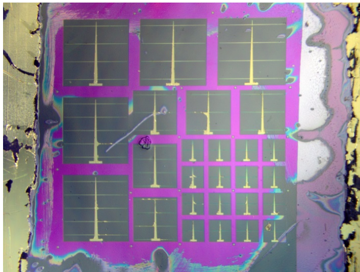
Figure 3.8: Top view of the device, transferred cell onto a flat Ag mirror.
