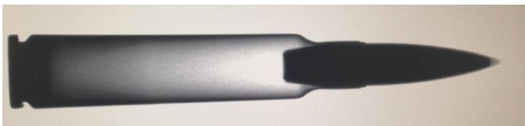
Figure 6 – Radiographic image of a cartridge using X-rays (Vattenhallen Science Centre)
