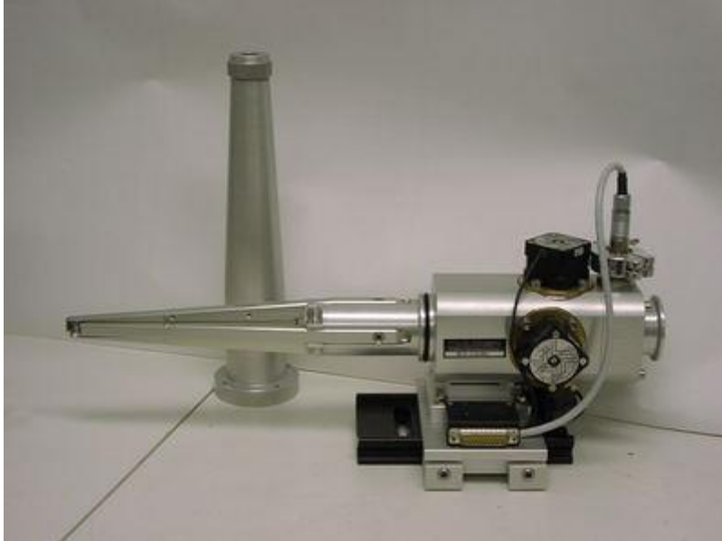
Figure 40 – Commercially available slit system provided by Huber, Vakuu Tube Cross Slit Screen 3002.60M (XMaS, ESRF)
