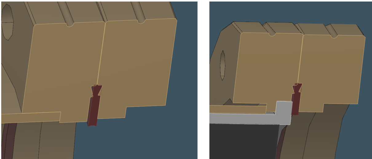
Figure 36 – The CF flange is used to lock the position of the Absorbing Baffles
