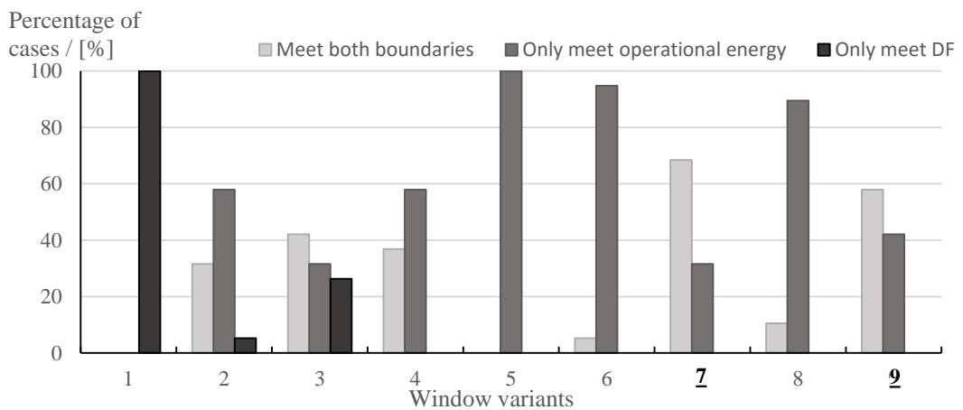
Figure 5-20. Percentage of cases (maximum is 19) which do meet or not meet the set boundaries for each window variant. Boundaries; annual operational energy of 20 kWh/m 2 and DF of 5 %.
