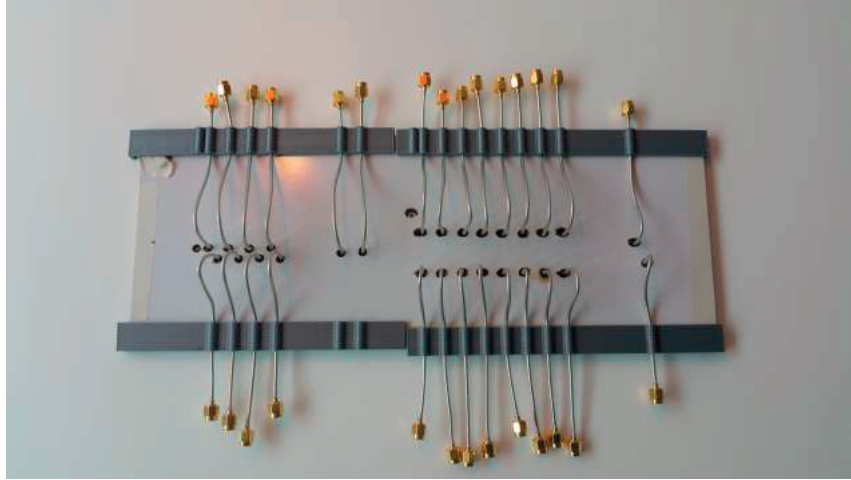
Figure 8.2: Picture of the backside with soldered rigid flex cables.
