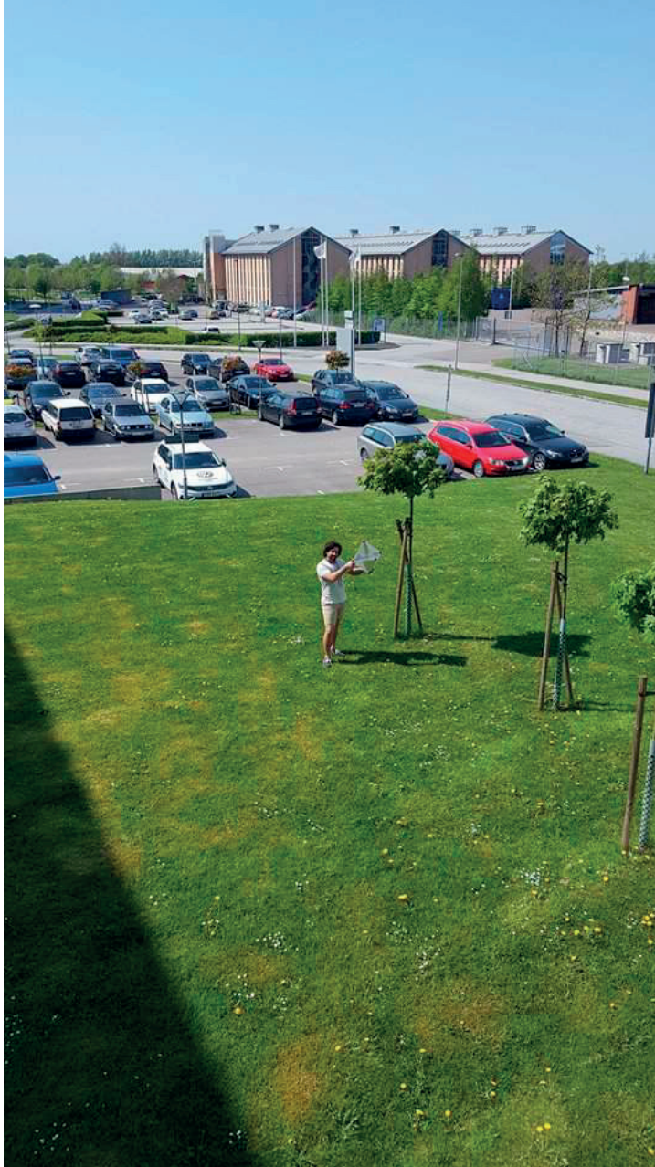
Figure 5.11: Picture of the area tested with the INRAS antennas. The person in the picture is holding up an octahedral radar reflector.
