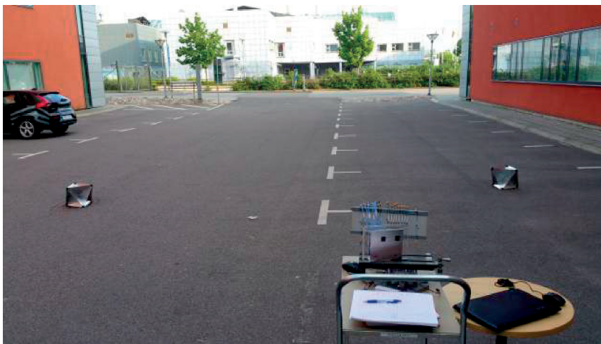
Figure 8.14: The second reflector located R = 5.3 m from the radar with an azimuth angle of \phi = 22^\circ and an elevation angle of \theta = 101^\circ relative to the radar.
