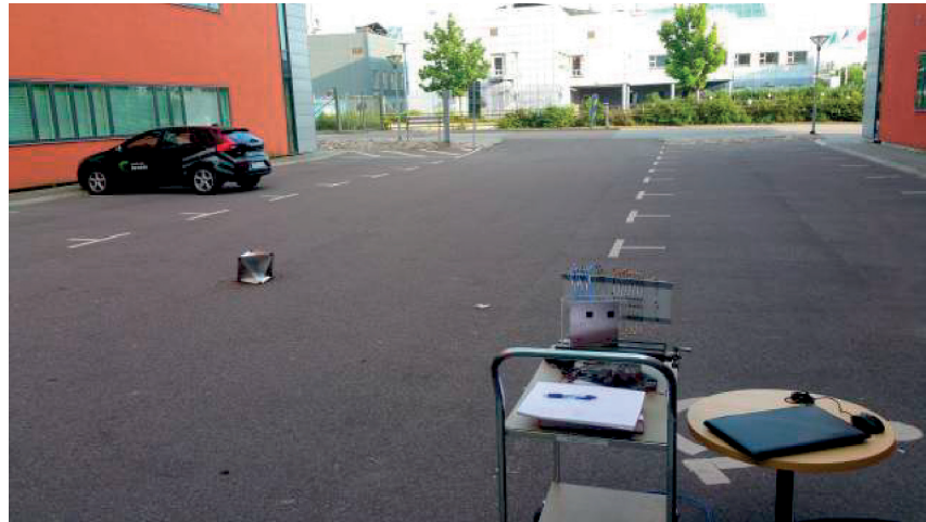
Figure 8.7: The reflector located R = 5.5 m from the radar with an azimuth angle of \phi = -43^\circ and an elevation angle of \theta = 100^\circ relative to the radar.
