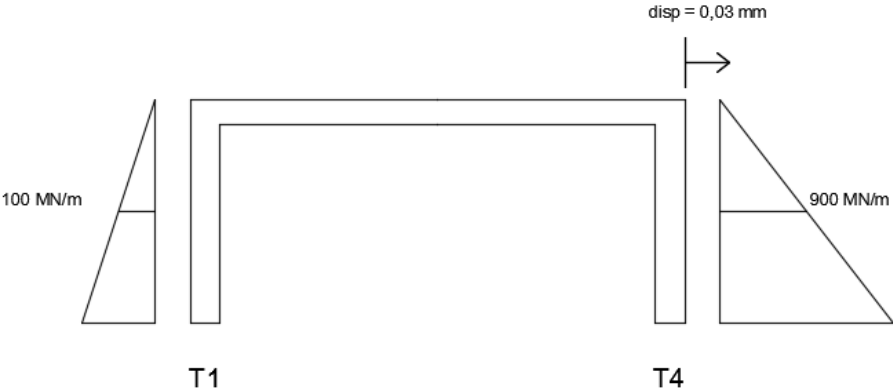
Figure 9.2. Iterated stiffness at the middle of the backwalls and the limit displacements for the braking of the crane.
