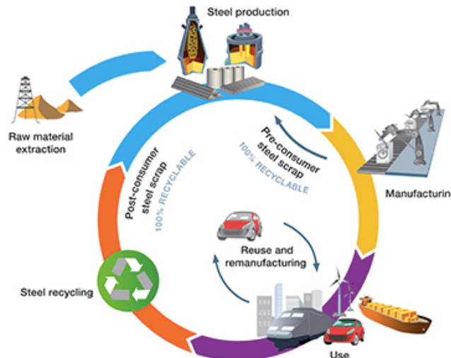
Figure 10. Flowchart illustrating the current life cycle of steel. Illustration from World Steel Association. 64
