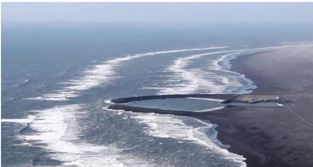
Figure 7: In front of the harbour entrance a gap in the bar can be observed where the waves are not breaking.
