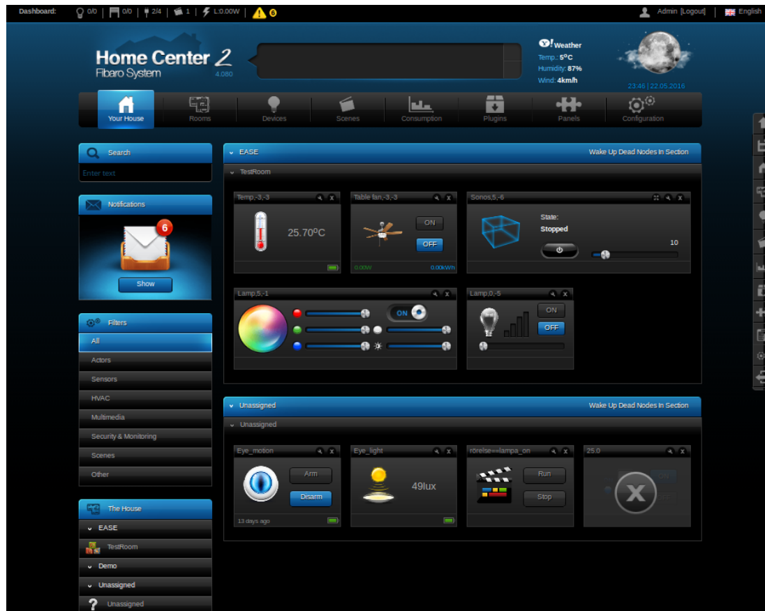
Figure 2.1: A typical Z-Wave controller web page (here the Fibaro Home System 2 administration page). The devices can be accessed in many ways e.g. depending on their type or location. The interface also offers scripting for automation. The device inclusion and exclusion are also managed here as well as more detailed device parameter settings.
