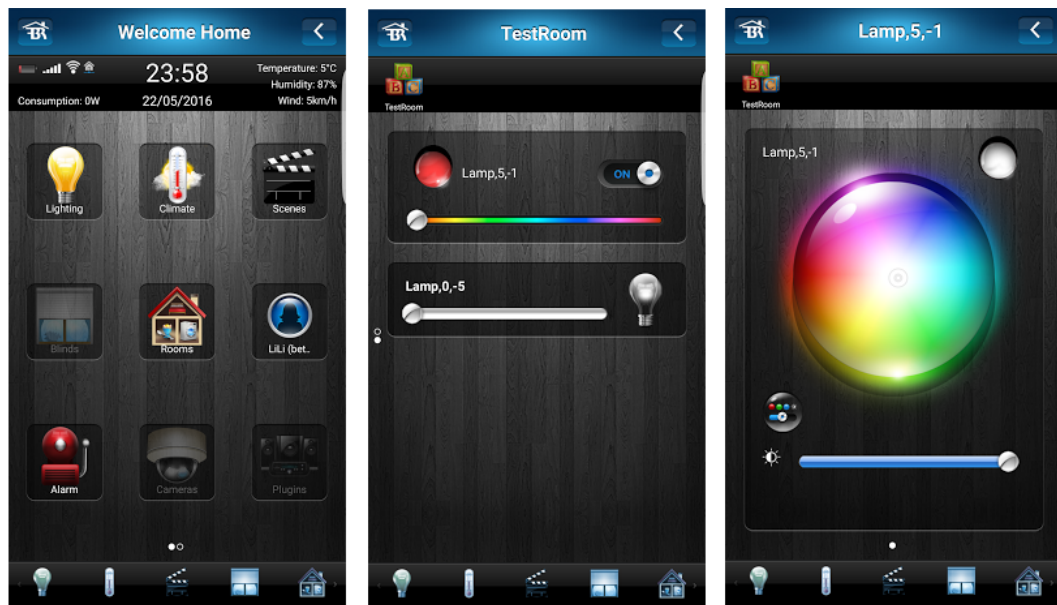
Figure 2.2: A typical Z-Wave controller mobile application (here an Android application from Fibaro). The devices can be accessed in many ways e.g. depending on their type or location. The interface is less advanced than the web page, but still offers some advanced operations. To the left, the main screen is shown. In the middle a specific room is selected and corresponding devices are shown. To the right, a dimmable lamp with colour adjustments is selected.
