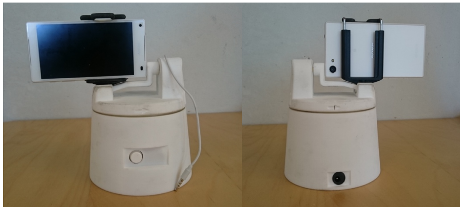
Figure G.2 - Left: Front side. Right: Back side. The phone must be placed properly so that the camera lens aligns with the rotating axes. Clamp the phone all the way back to the attachment and push it as far to the right as possible, viewed from the front.
