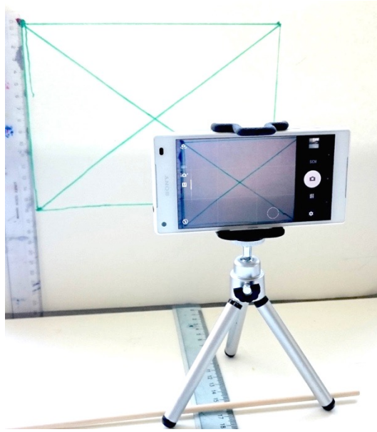
Figure 5.5 - Measuring the field of view of a Sony Xperia Z5 Compact
