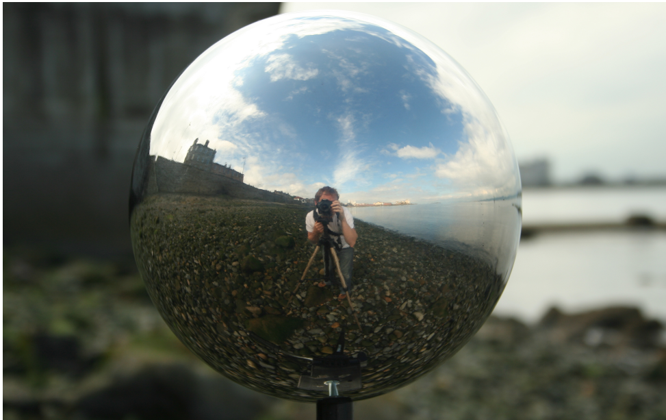
Figure 2.1 - Photograph of a spherical mirrored ball, sometimes used in IBL [7]
