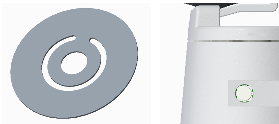
Figure 9.11 – Left: the spacer with the circular guiding track. Right: The acrylic spacer assembled between the top and bottom part.
