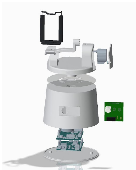
Figure 10.3 - Exploded view of all the components in the final product.
