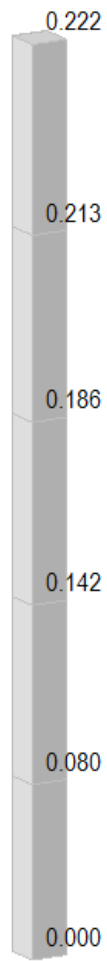
Figure 6.27: Deformation [mm] of column without construction stage analysis. Dimensions are 1x1x25 meters.
