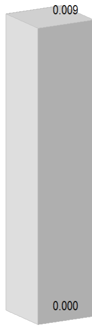
Figure 6.24: Deformation [mm] of column at first construction step. Dimensions are 1x1x5 meters.
