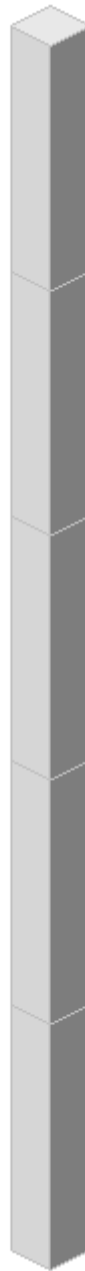
Figure 6.23: Model of concrete column to demonstrate deformations with construction stage analysis. Each section of the column has a width and depth of 1 meter and a height of 5 meters, giving a total height of 25 meters.
