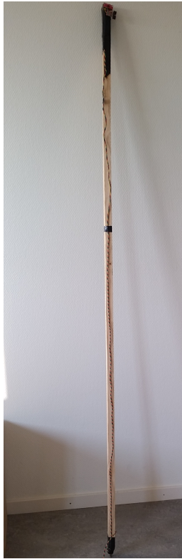
Figure 7.1 Sensors are mounted at the top of the stick. The stick is approximately 2m long.
