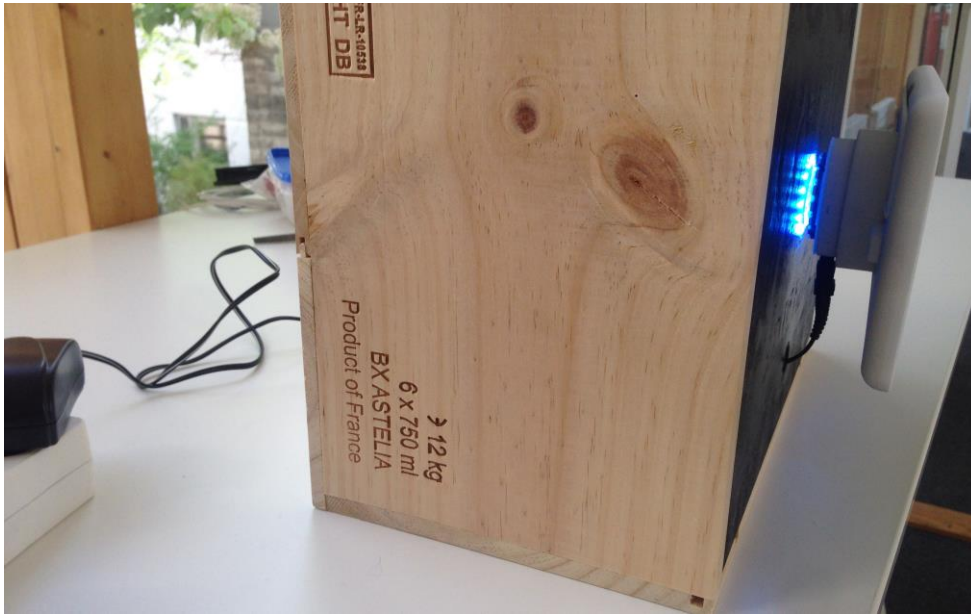
Figure 11.3 Sideview of the complete prototype docked and charging on the demonstration box. Also seen in the image is the power adapter(left).
