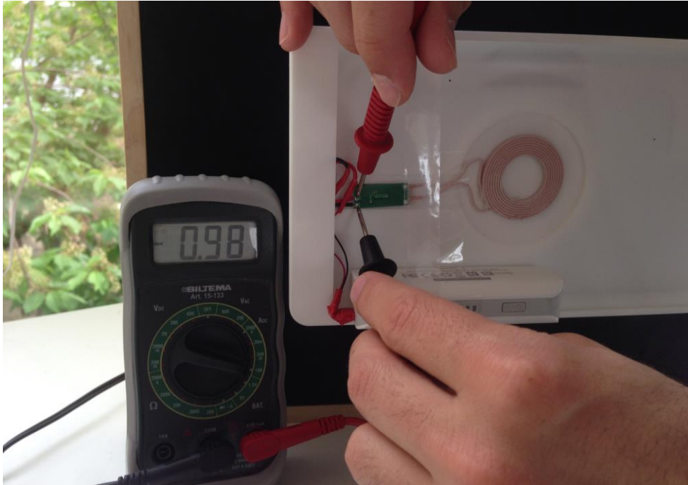
Figure 9.4 Testing the electric current flowing into the battery. Results are showing 980mA.
