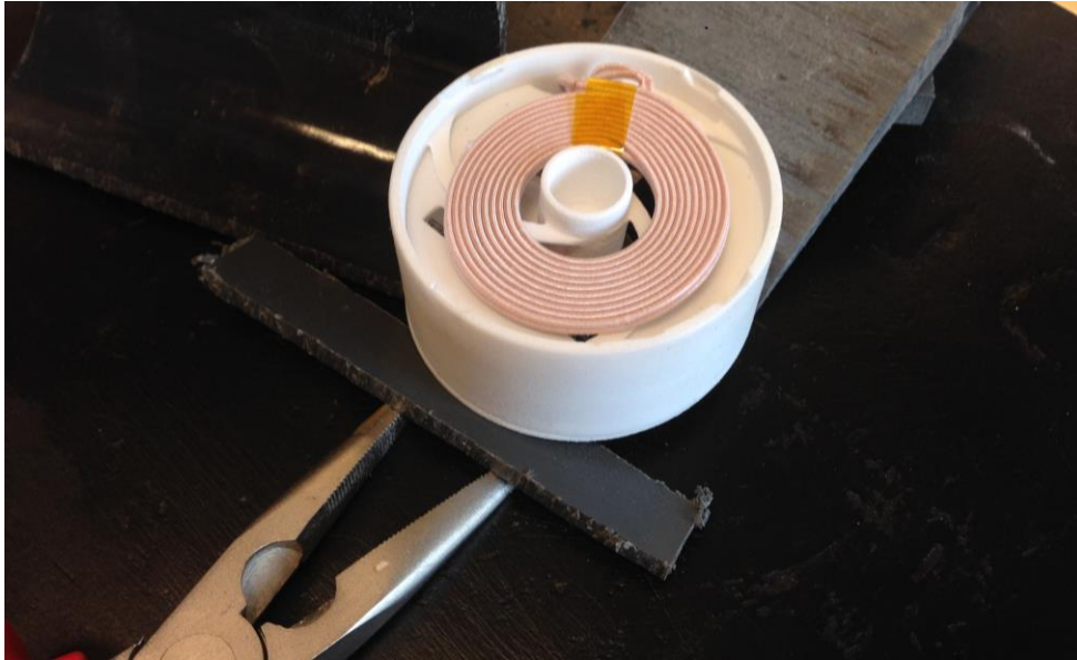
Figure 8.41 Glue together the shell with the base because the designed snap-fits weren't strong enough to hold it together.
