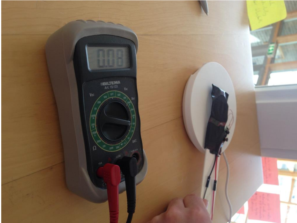
Figure 7.5 Testing the prototype receiver with the wireless charger from IKEA and seen with the multimeter that there were little, or no, current flowing. (8mA)
