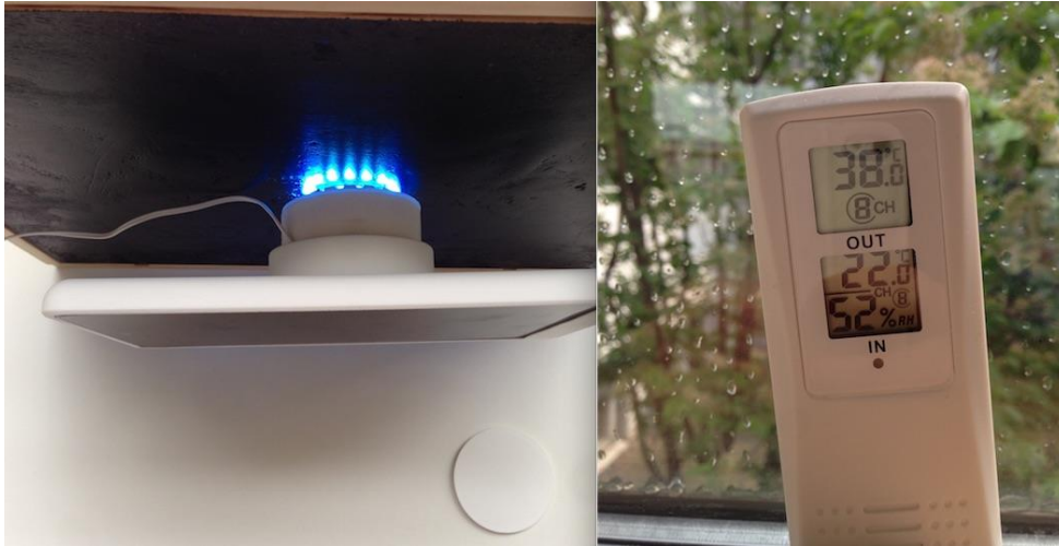
Figure 9.6 Measuring temperature inside the PUCK.
