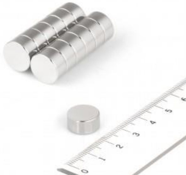
Figure 8.1 Neodymium magnets close to a ruler indicating their size. Image reference [17]
