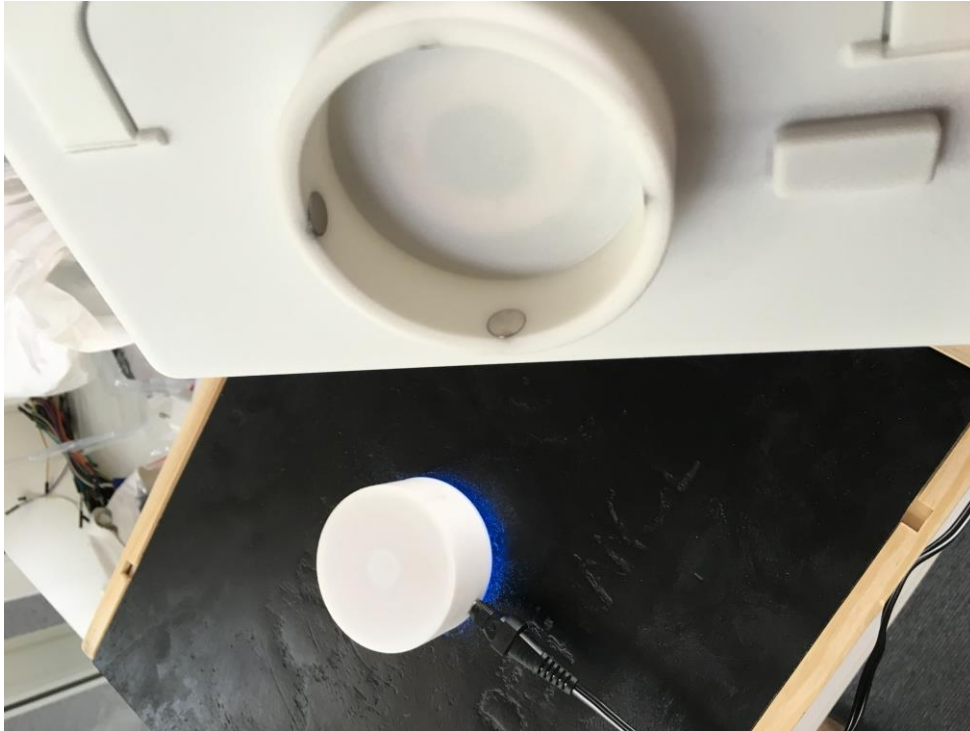
Figure 8.40 Outside of the puck (Lower) and inside of the ring (Upper) after surfaces has been sandpapered.
