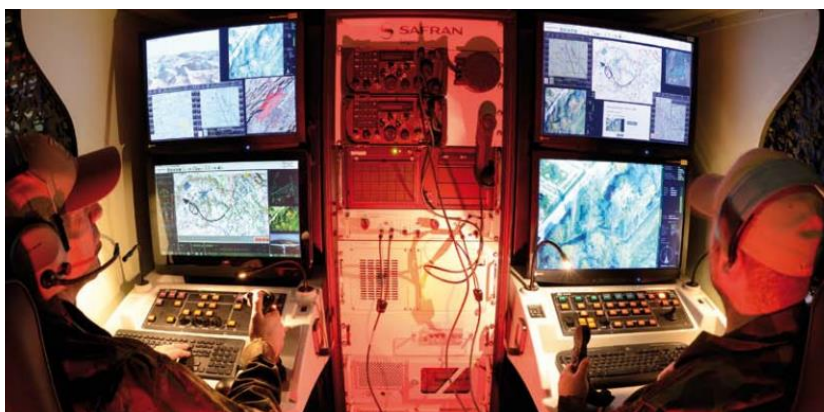
Fig. 2 - Ground Station, on the left the UAV operator and on the right the payload operator
