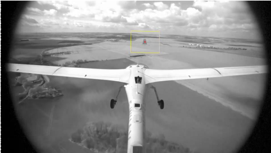
Fig. 10 - Tracking Algorithm view, the red cross is the tracked point, the TDP, and the yellow square delimits the image analysis area
