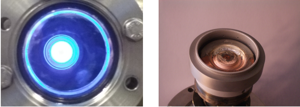
(a) Magnetron sputtering source in action. (b) Magnetron with 2 inch diameter silver target.
