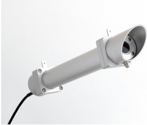
Figure 3. The picture shows a pyrheliometer, which is used for measuring direct solar radiation. During the measurements the instrument is directed towards the sun (Goswami, et al., 1999)
