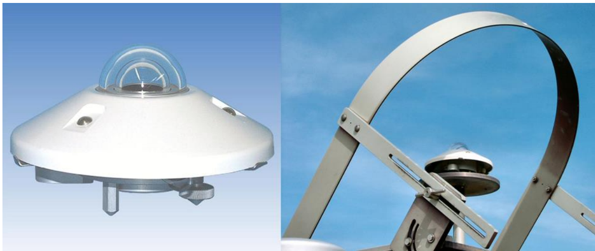
Figure 2. The image to the left shows a typical pyranometer, which is used for measuring global solar radiation and diffuse solar radiation. The image to the right shows a shadow band placed around a pyranometer in order to exclude the direct sunlight from the measurement.
