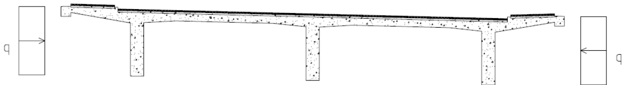
Figure 12. Figure illustrating how the vertical global solar radiation acts at the southern and the northern side of the bridge.
