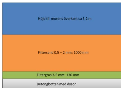
Figure 5-4: Schematic diagram for the 25 filters (Persson, T., et al, 2015)
