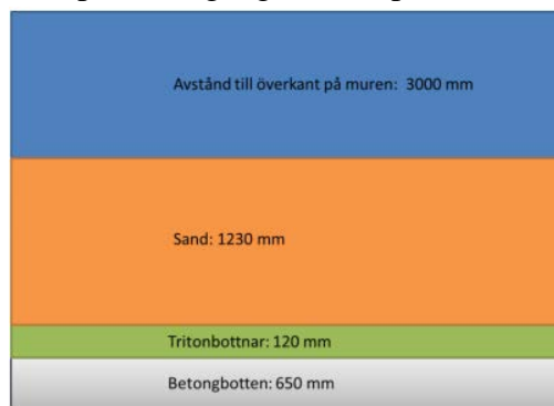
Figure 5-3: Schematic diagram of the filter 2. (Persson, T., et al, 2015)
