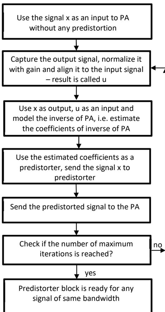
Figure 4-3: Flowchart of DPD algorithm
