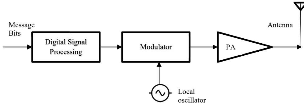
Figure 1-1: Block diagram of a simplified modern transmitter architecture
