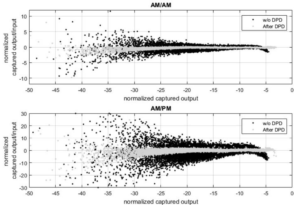
Figure 5-8: Comparison of AM/AM and AM/PM curves without DPD and after DPD
