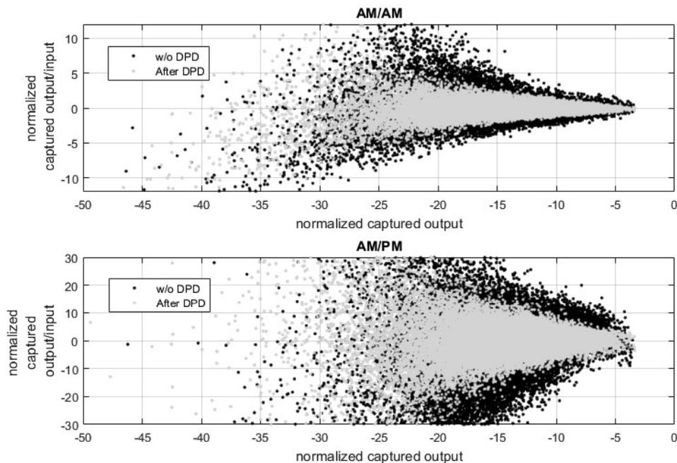
**Figure 5-6: Comparison of AM/AM and AM/PM curves without DPD and after DPD**
