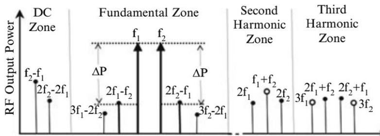
Figure 1-8: 2 tones test results of a PA, when the PA is in non-linear region [10]
