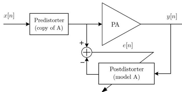
Figure 4-2: Basic schematic of digital predistortion of a power amplifier [26]
