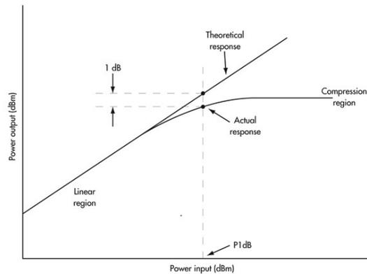
**Figure 1-5: Input power vs output power for 1 dB compression point**
