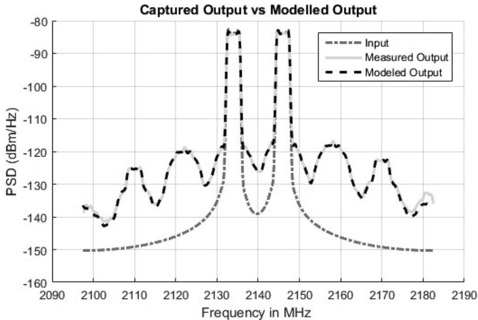
Figure 5-4: Input, captured output and the modelled output for ACRSV method
