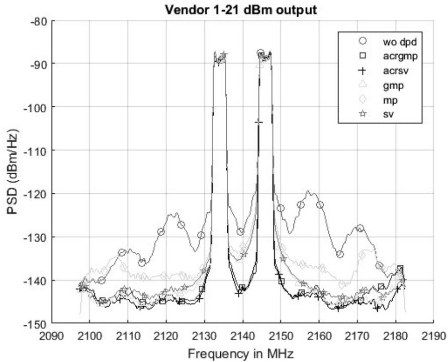
Figure 5-5: Frequency spectrum of output of the PA from vendor 1 after DPD, for 21 dBm output power
