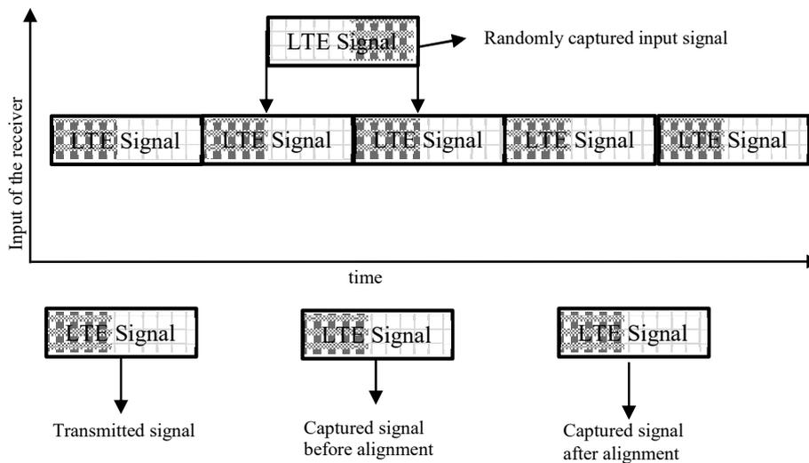
**Figure 3-4: Diagram of received and captured signal before and after alignment**
