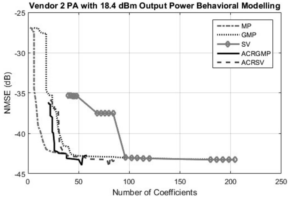
Figure 5-2: Number of Coefficients vs NMSE for 5 different behavioral modelling methods
