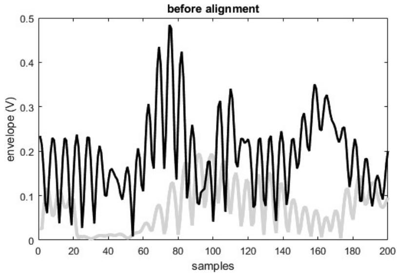
Figure 3-5: input and captured output before alignment
