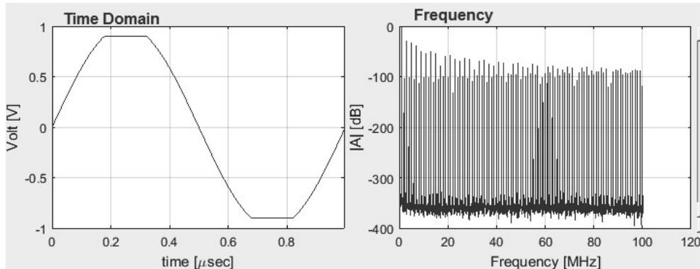
Figure 1-7: 1 MHz Sinusoidal wave with clipping & its frequency response
