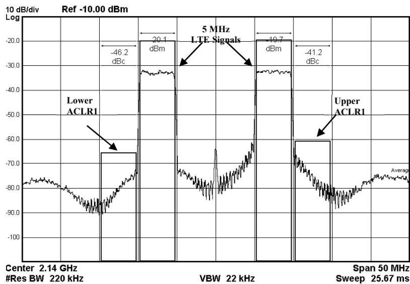
Figure 1-4: ACPR1 regions for 2 cascaded 5 MHz LTE signals with 15 MHz spacing
