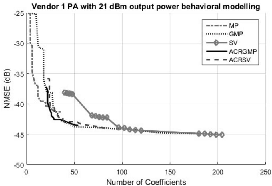
Figure 5-1: NMSE vs Coefficients number for 5 different methods, for behavioral modelling
