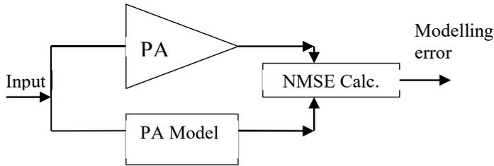
**Figure 3-3: Schematic of the comparison method after modelling the PA**
