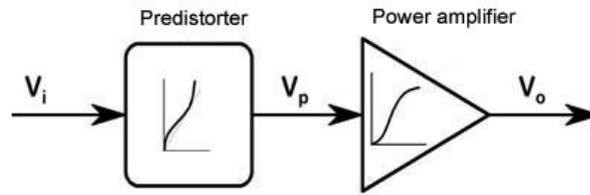
Figure 4-1: Inverse transfer function of a power amplifier placed before the power amplifier
