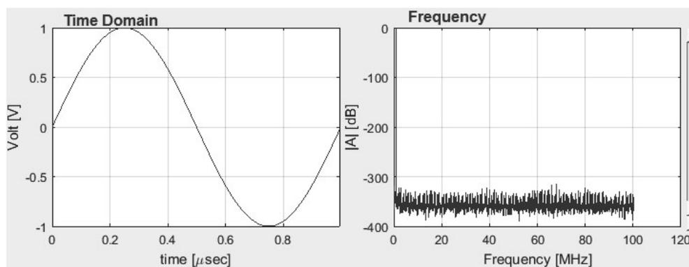
**Figure 1-6: 1 MHz Sinusoidal wave without clipping & its frequency response**
