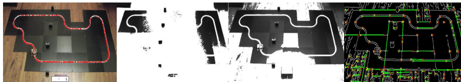
Figure 55: A comparison of the line detection algorithm developed during this project (most left image) and three other commonly used algorithms. From left: In project developed algorithm, fixed value thresholding, Otsu thresholding and Hough line transform.
