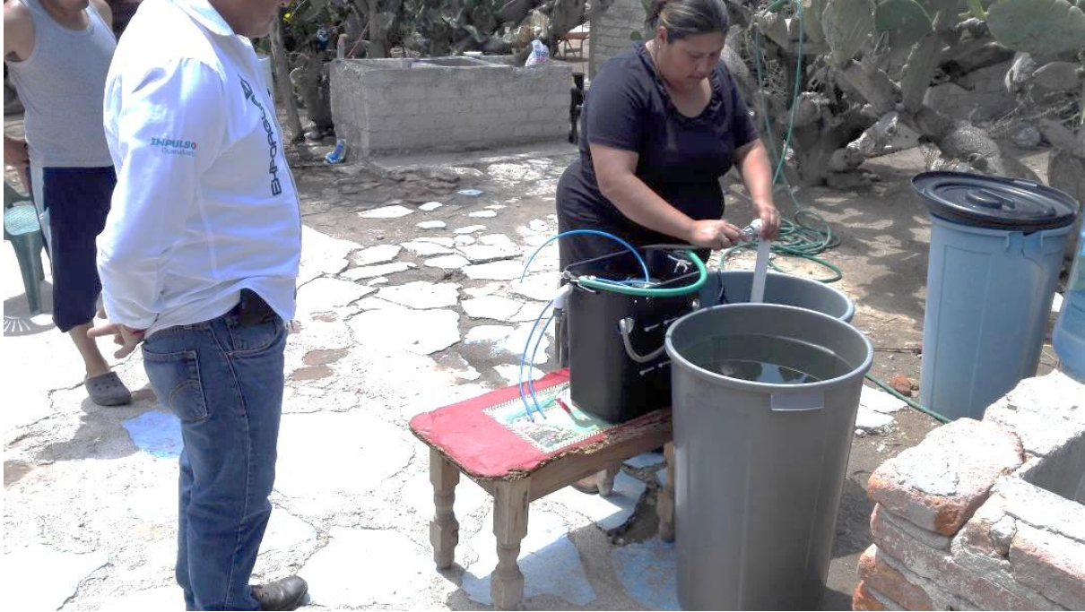
Figure 4-9 Shared reverse osmosis filter being used at La Cinta
