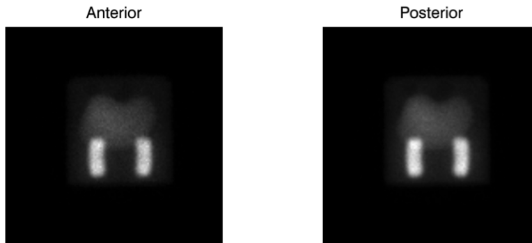
Figure 17: Anterior (left) and posterior (right) images of the KYOTO KAGAKU phantom filled with activity as shown in table 5.
