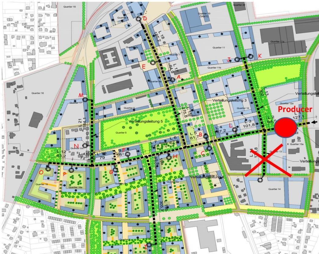
Figure 27 - District heating network for a small area in Graz. Picture taken from (TU-Graz, 2015).
