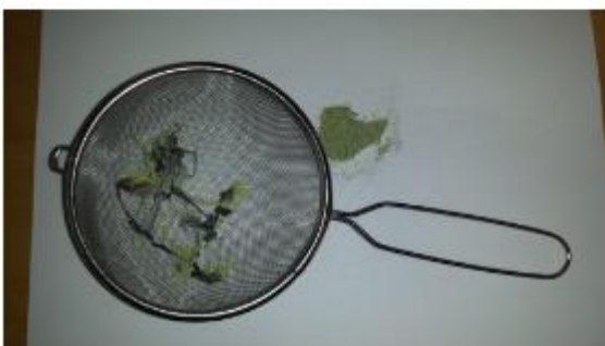
fig 6.1.5 Plastic granulate from belt sander, the granulate was mainly from the cork
