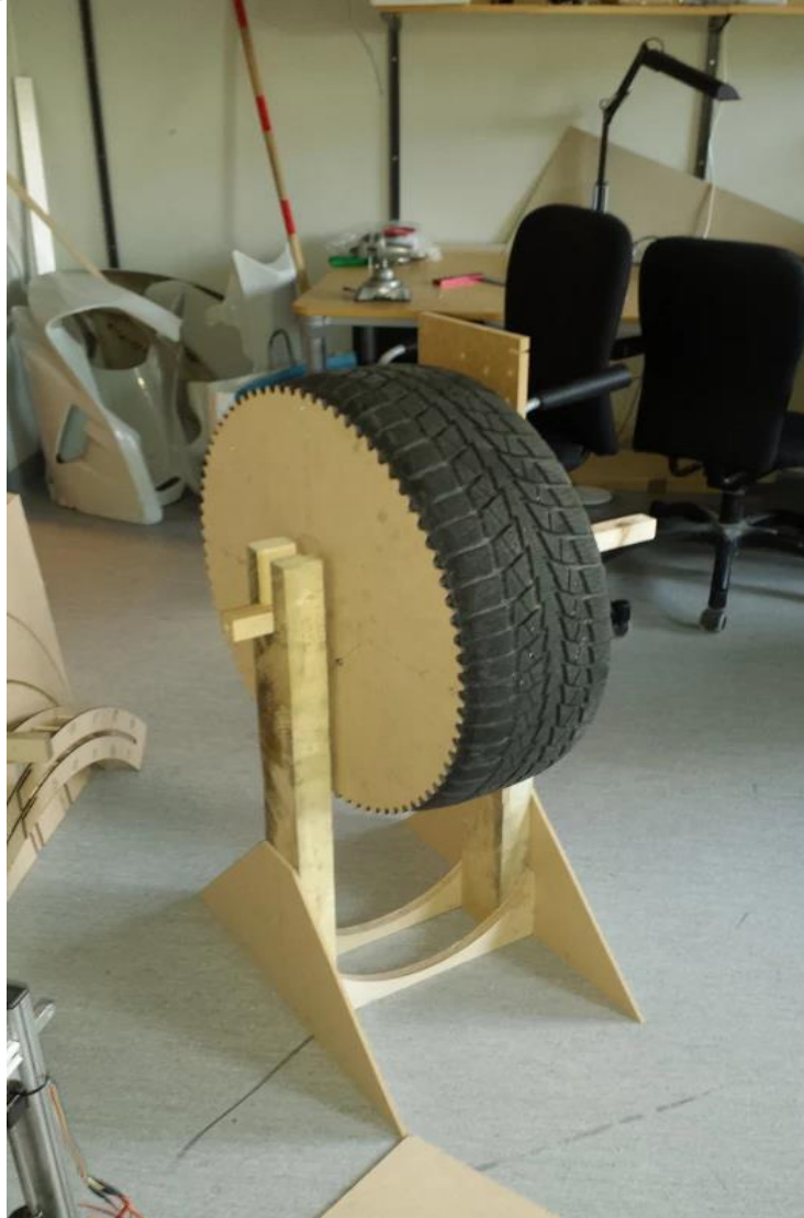
fig. 2.6 Iteration 5: Peripheral Direct Drive
