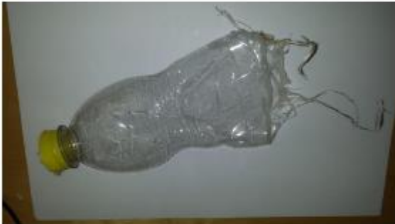
fig 6.1.3 Bottle after belt sander test
