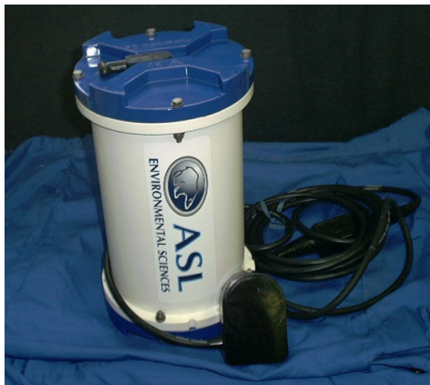
(a) Image of the Zooplankton Acoustic Profiler (ZAP) by Lemon et. al. [13]. (b) Data from ZAP, showing the diel vertical migration of zooplankton. Image from [14].
