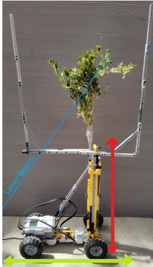
Figure 5.15: A simple robot was constructed for smooth moving of the plant. A period consisted of a forward and backwards movement across the laser beam before the plant was raised 0.5 cm and the process repeated.
