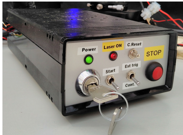
Figure 3.6: The physical control box for the laser, constructed by Igor Buzuk.
