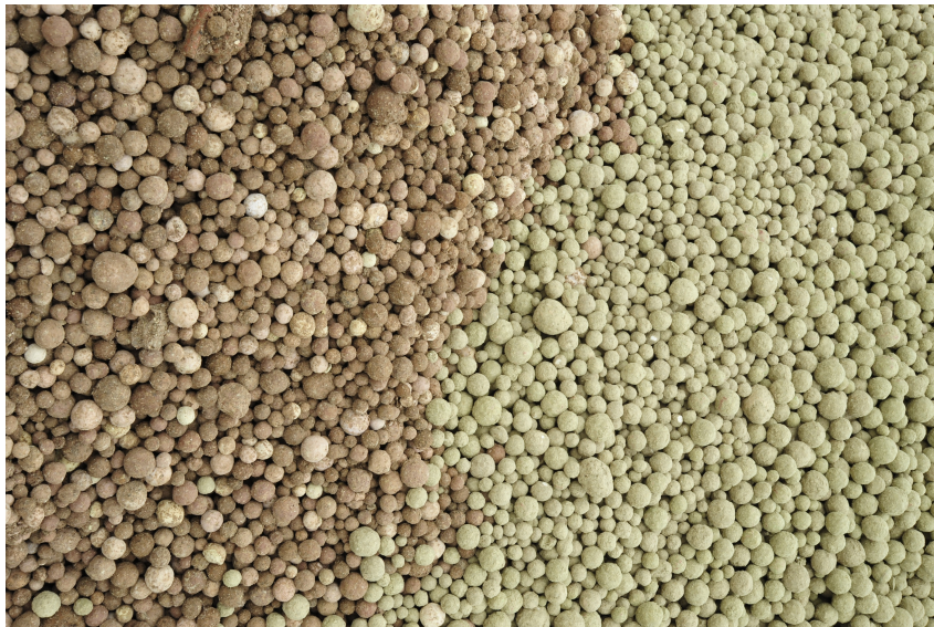
Figure 3.1.: LWA 1 used at a landfill in Landskrona
