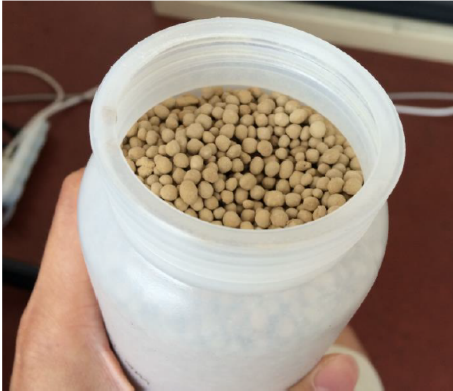
Figure 3.2.: LWA 2 manufactured in laboratory
